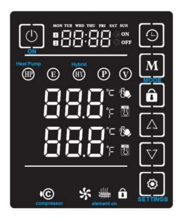
The SunPump 3.1 uses the following indicators to display system status.
