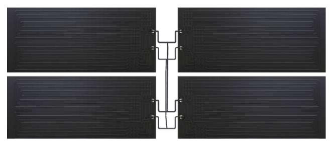
This is a 4-panel array sample configuration which may vary depending on installation parameters. A South exposure and 30 to 90-degree angle is needed. Alternatively, an East/West split of panels works well. In high snow locations consider wall mounting under the roof overhang, or very steep angles to avoid snow and ice accumulation.
