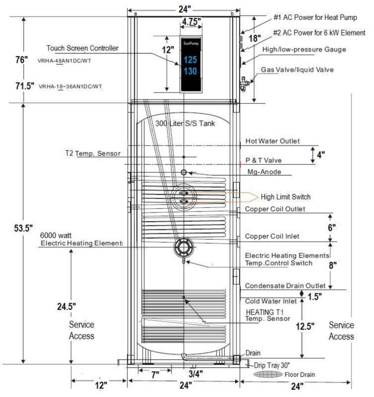
NOTE: All Water, Refrigerant and Electrical connections are on the right side, allow for service room to left and right.
