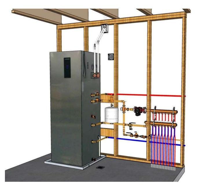
The 3D scale model show above, is typical of a radiant floor and domestic hot water installation. Your distribution system may be different, it could use an Air Handler and ducts to distribute heat as an alternative.
