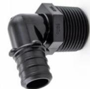
c). If temporary, use a 3/4" brass plug in the port marked Cold Water In. Alternatively install a permanent elbow like the 3/4" PEX x MIPT at right. Design flow rates are 2.5 GPM per 3.5 kw or 12,000 BTU. A 14 kw will require a 1" pump that provides  $14/3.5 = 4 \times 2.5$  GPM = 10 GPM at 10-15 Feet/Head.
