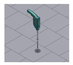
Make sure the sealing washer is positioned correctly on the threaded shank of the Aluminum Shoe Use roofer bar to lift roof shingle, slide the flashing under shingle, and insert the flashing over the threaded shank.
