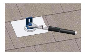
Install AL rail to "L" foot to the specific orientation. Then, tighten
